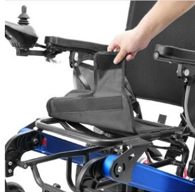
The seat strap is fixed by Velcro, which is easy to disassemble and assemble.
